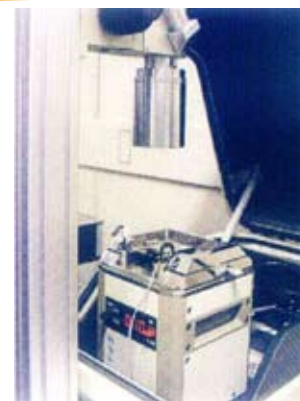
Positioning of FE300 on top of see through glass of vacuum chamber
