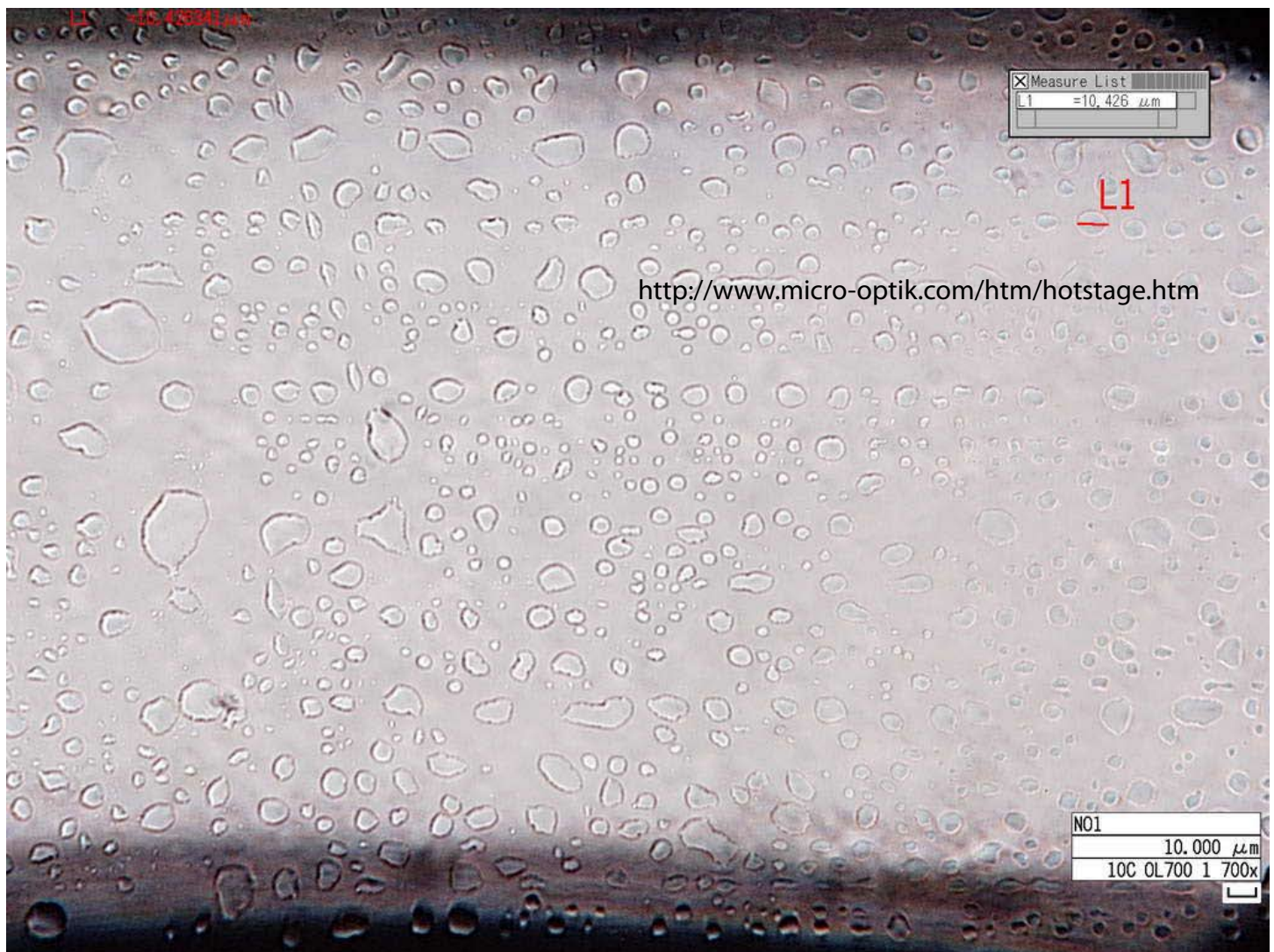
Figure 3 Microscopic image of the surface of a bicomponent PP/PE fiber with liquid dispersed on the surface, recorded with Microptik K3000 Digital microscopic analyzer with 10C OL 700 lens. Magn = 700x.
